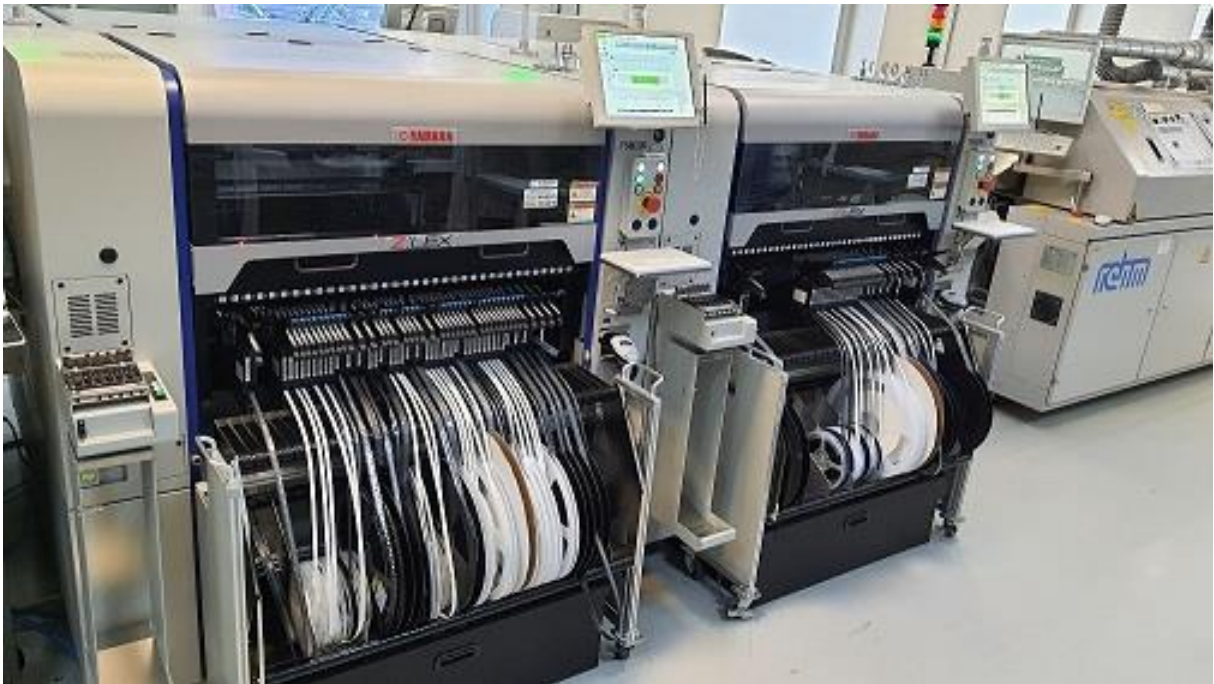
Figure 1. The two YSM20R mounters work in series to maximise throughput and flexibility.
