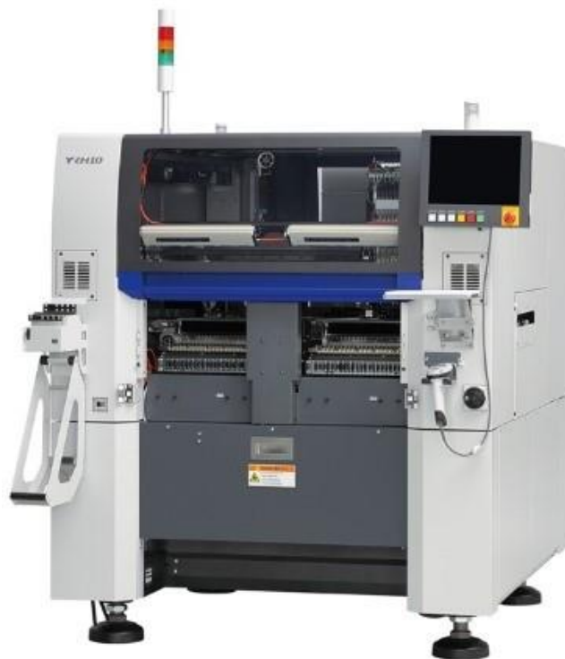
Figure 3. The YRH10 hybrid flip-chip bonder and surface-mounter launched in 2021.
