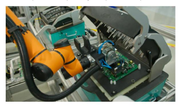
To meet these challenges, **KINALI** and **ATX Hardware HmbH** have joined forces. By combining the **Test-it-off** automation platform from KINALI with **ATX automatic opening and closing (AOC E/P) fixtures**, a next-generation automated PCBA testing solution is born. Their integrated solution follows **Industry 4.0** principles and moves manufacturers closer to fully automated, Dark Factory-ready production.
