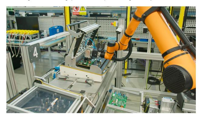
Producing around **400,000 PCBAs annually**, BTL operates in a **High-Mix, Low-Volume** environment where flexibility and precision are essential. Manual testing limited throughput and scalability, while frequent product changes required constant reconfiguration. To address these challenges, BTL implemented the modular **Test-it-off** platform, which automates testing, reduces manual handling, and enables autonomous operation.
