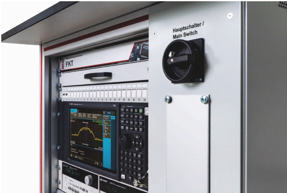
Picture 2: Spectrum analyzer during the process of testing WiFi and ZigBee signals
