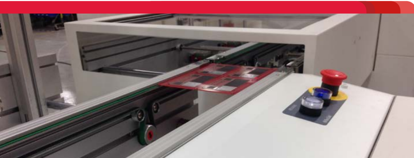
The "open transfer" belt driver system eliminates shafts and bellows by incorporating a dual motor, ESD safe belt system.
