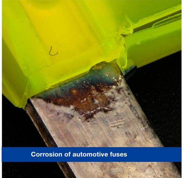
Corrosion of automotive fuses
