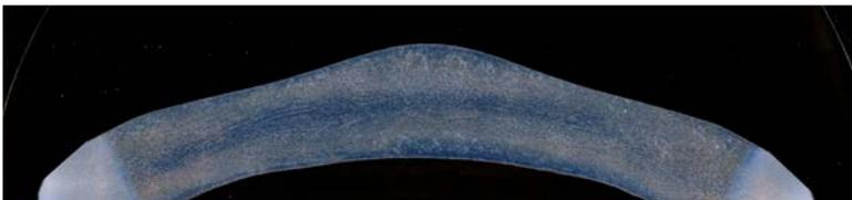
Cross-section of engine valve
