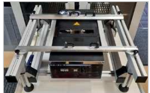
EXAMPLE OF A CUSTOMISED PRINTED CIRCUIT BOARD MOUNTING FRAME FOR HEAVY AND LARGE ASSEMBLIES. CIRCUIT BOARD CAN BE MOVED IN X-DIRECTION. Y-AXIS COMPLETELY MOVABLE.
