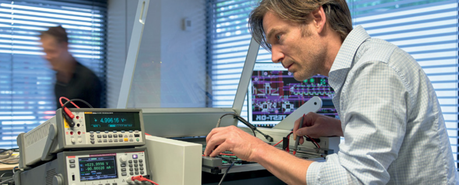
Verification of aTCC-controller card in the TEST-OK System
