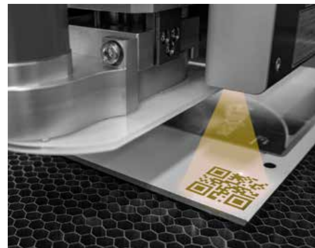
Automated QR code recognition and selection of job data with JOBIDENT
