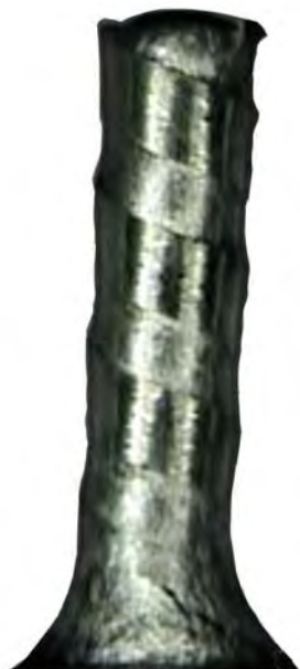
Free end Solder Bump Before Planarizing
