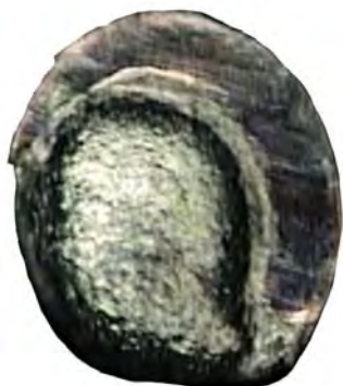
Solder Bump Top of Column
