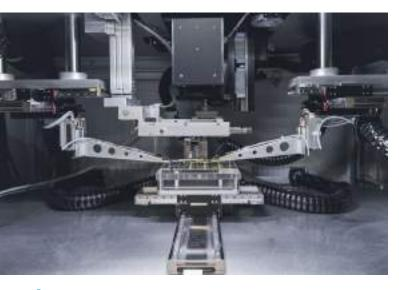
EXAMPLE OF PROBING SYSTEM WITH 3 FLYING PROBES (WITH ACTIVE PIN GUARD MODE)
