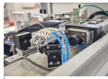
DIODE PUMPED GENERATOR INFRARED (1064 nm) or GREEN (532 nm)
